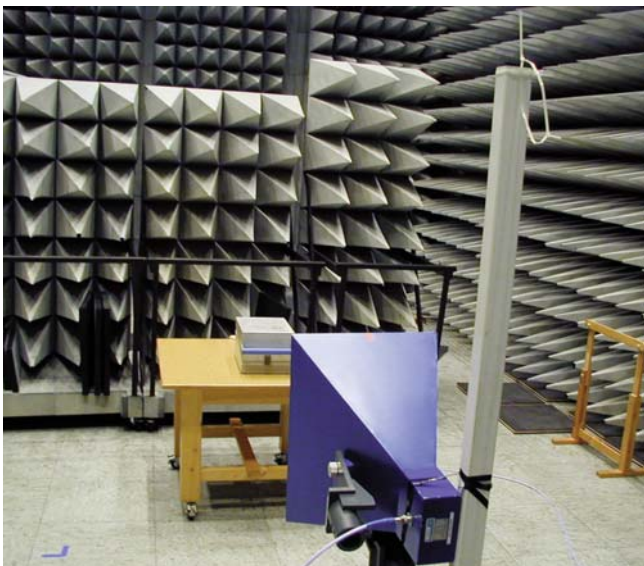
4921 RF Shield with transmitting antenna in EMC laboratory
