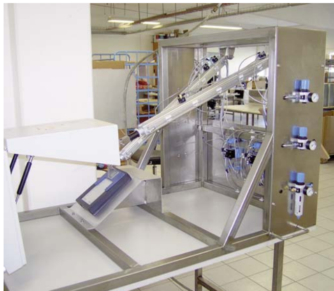
Mechanical life test of the 4921 RF Shield
